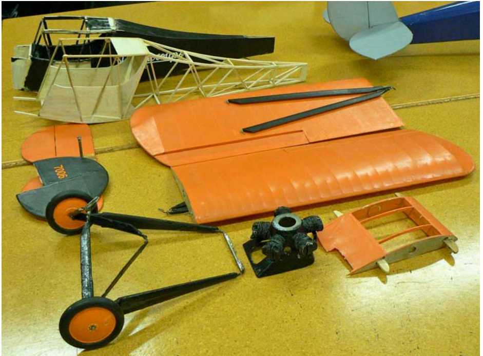
Above: Stan Mauger's Monocoupe Velie fuselage is being rebuilt to create a lighter model.
